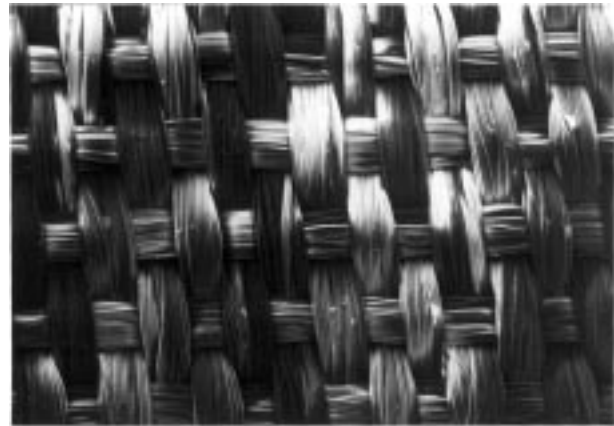
Figure 2 Photomicrograph illustrates knitted poly(glactin) mesh organization (SEM original magnification \times 50 ).
